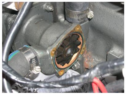
Besides the water pump impeller, I changed the oil, installed a new fuel filter, and a new V-belt on the engine.
