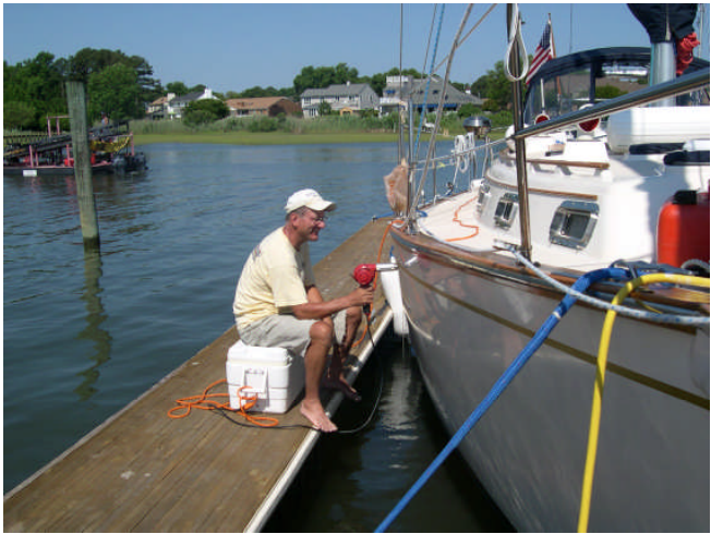
Roy with a heat gun on the hull to remove the old stripe.
